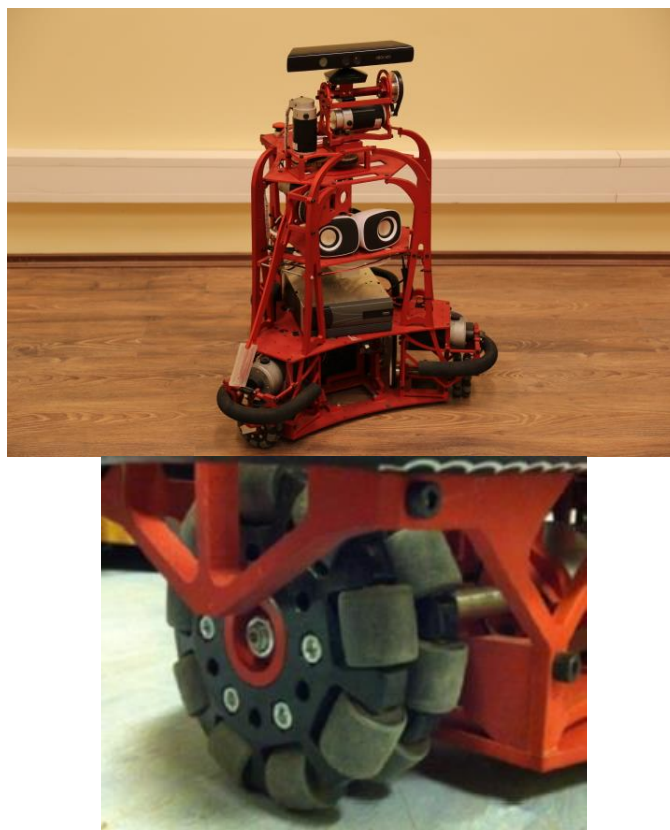
Fig. 1. The Ethon robot (left) and its holonomic wheel (right).
